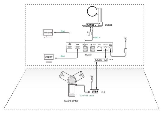
The IP phone should be powered by PoE adapter (54V/0.56A) or PoE switch. All devices are powered separately. The cable should be replaced at once if its skin is broken.
